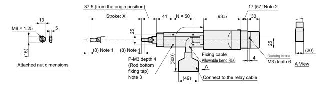
Note 1: Operating range during origin return Note 2: The numbers within the [] are the dimensions with the brake
