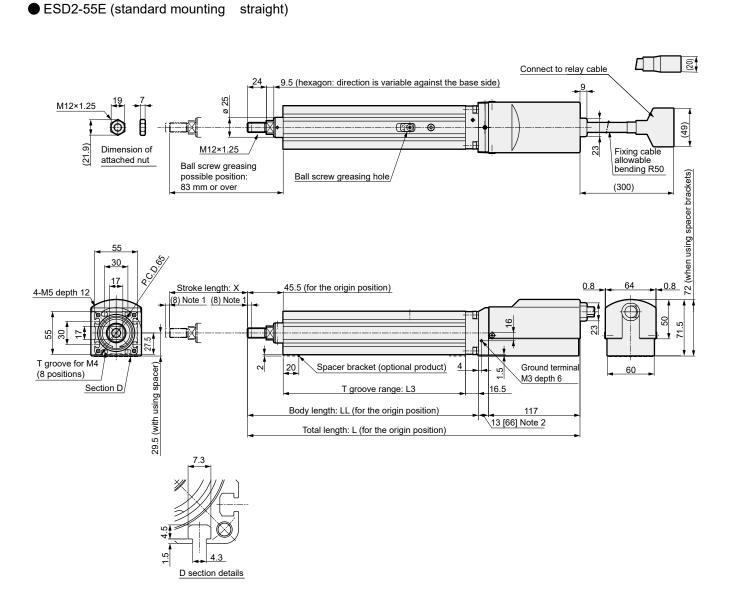
Note 1: Operating range during origin return Note 2: The numbers within the [ ] are the dimensions with the brake
