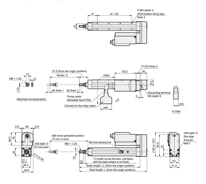
Note 1: Operating range during origin return Note 2: The numbers within the [] are the dimensions with the brake
