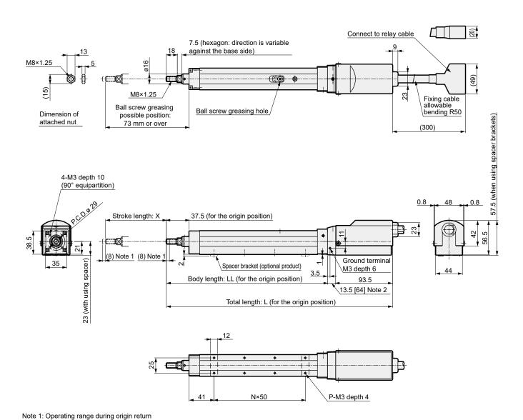
Note 2: The numbers within the [] are the dimensions with the brake
