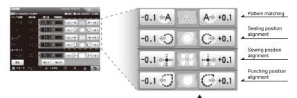
Position alignment can be easily set with "+" and "-"
