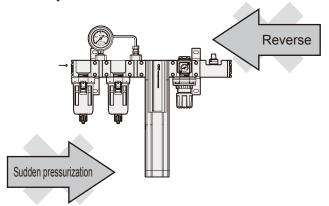
■ The oil mist filter life is spent when the pressure drops to 0.07 MPa or after one year of use, whichever comes first. Replace the mantle with a new one at the end of its life (check the pressure drop with a differential pressure gauge). (Do not touch the urethane rubber foam layer when replacing the mantle) [NSU Series]
