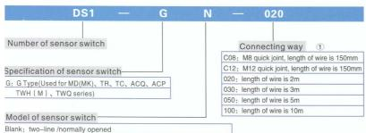
$N{:}\ \ three-line \ NPN \ with \ no \ contact \ (current \ flows \ in)/ \ normally \ opened$   $P{:}\ \ three-line \ PNP \ with \ no \ contact \ (current \ flows \ out)/ \ normally \ opened$
