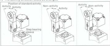
2. The rolling wheel could be installed at the inside of leverage
