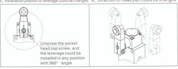
5. Length of contact pin could be changed
