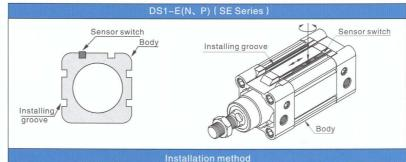
Adjust the clamping screw on sensor switch to the parallel position that enables the sensor switch to enter the installation slot. Then lead the sensor switch to the installation slot and adjust it to the proper position and tighten the clamping screw to fix.
